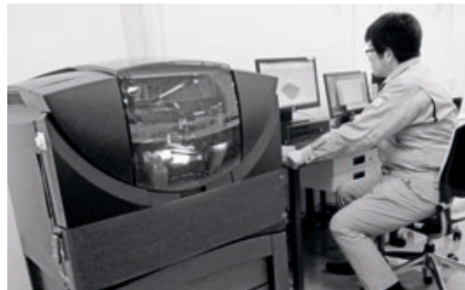
Three-dimensional printing technology used to produce surgical templates at Straumann's new CAD/CAM center in Japan.
