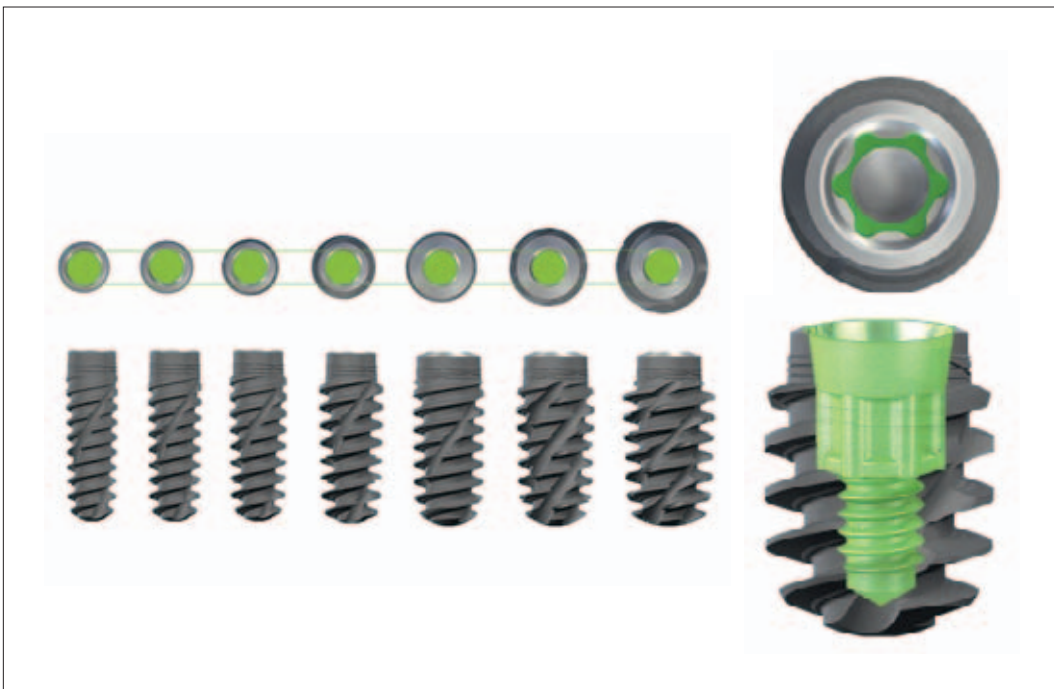
Fig. 11 Detail of the Torc Fit® connection: the connection is the same for all implant diameters, its internal configuration allows six positions, an internal Morse tapered angle of 7°, guaranteeing the seal of the connection, and an external bevel, oriented at 22.5°, with a polished surface. Finally, the reduced height of the Torc Fit® connection of 5 mm reduces the minimal implant length to 6 mm.
