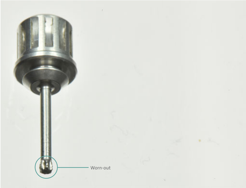
Fracture of a Torque Control Device
