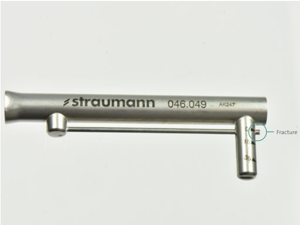
Fracture of a Torque Control Device
