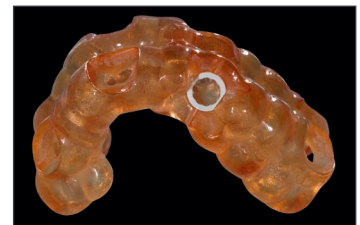
The guide is printed and the sleeve is glued into place
