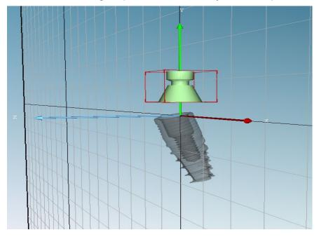
Create Implant Libraries - Instructions Optional components Before creating the implant kit, STL files must be placed in the same referential coordinate system, along the vertical (Y) axis with the center of the head of the implant positioned at 0x0x0.
